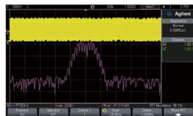
KEYSIGHT DSOX2000A - FFT Display
